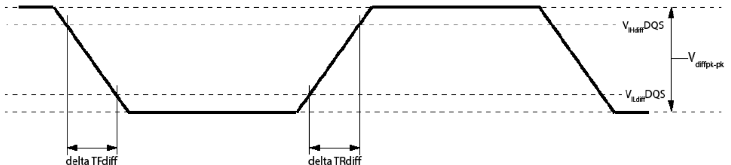
Figure 14 – Differential Input Slew Rate Definition for DQS_t, DQS_c
